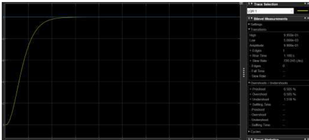
Gambar 9.14 Hasil Simulink Motor DC M66CE-12 LQR tanpa noise
