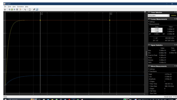
Figure 8. Comparison of Responses for Brushless DC Motor 866BLF03 with and Without LQR Method
