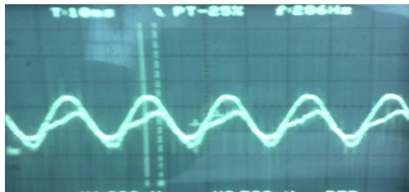
Figure 4. The input voltage and current waveform for the load constant for V_s = 15 Vrms
