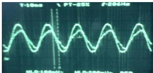
Figure 5. The input voltage and current waveforms for constant load for V_s = 17 Vrms.
