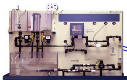
Figure 2. Level and Flow Process Rig 38-100
