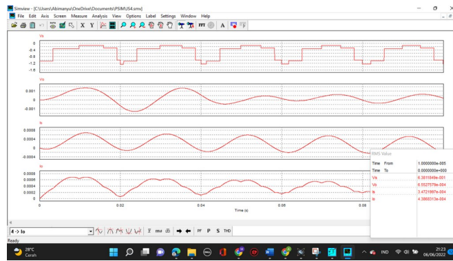
Figure 10. rms waveform of experimental rectifier 3 with a 60 v
