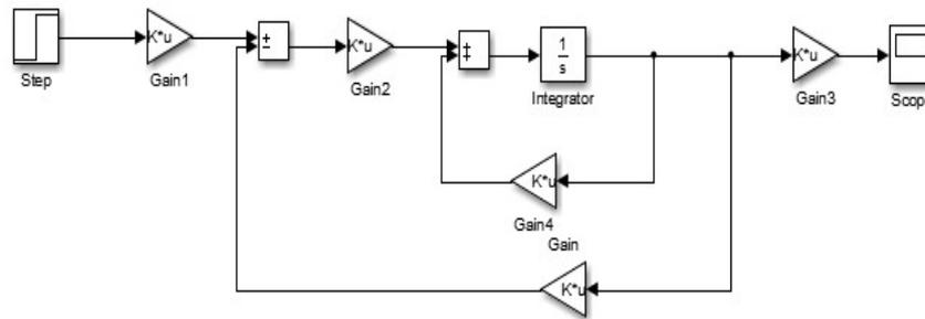
Figure 5. SISO Modeling Using LQR
