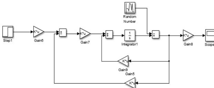
Figure 2. SISO Model DC Motor with LQR and Noise
