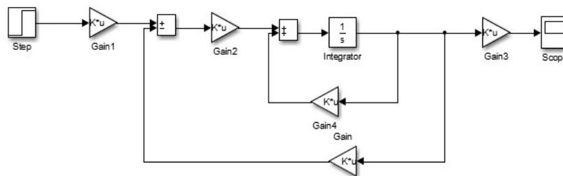
Figure 1. SISO Model DC Motor with LQR
