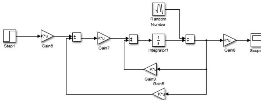
Figure 6. SISO Modeling with Noise Using LQR
