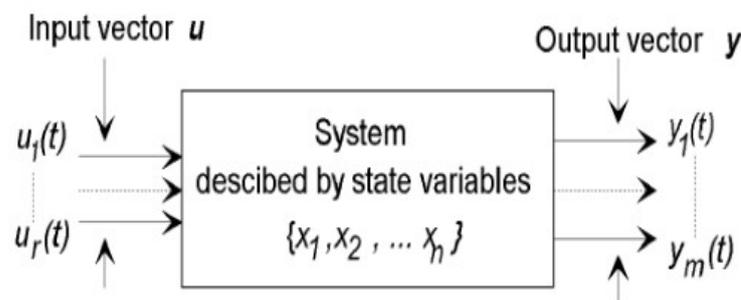
Figure 4. Input and Output Systems in State-Space
