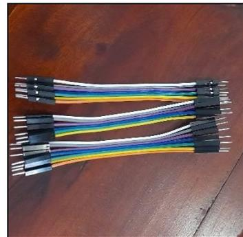
Gambar 13. *Kabel Jumper*
