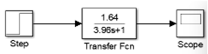
Fig. 2. Open Loop Block Diagram of 1st Order Baldor L3510 1 Phase AC Motor
