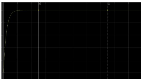
Figure 8.Response Results of the PG36M555 DC Motor Using the LQR Method
