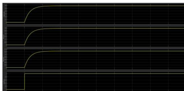
Figure 11. Response Results of the PG36M555 DC Motor Using the LQT Method
