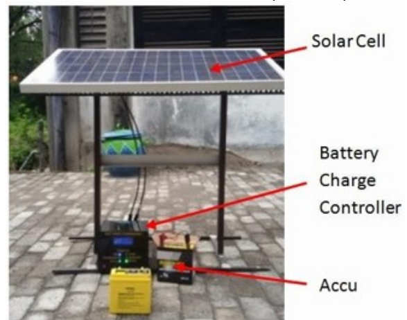
Gambar 4.5 Instalasi Pengujian sistem baterai charge controller
