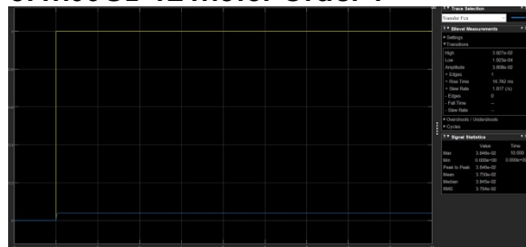
Figure 3.3 LQR Step Response Display In Figure 3.3, there is a blue graph that has not reached the set point. The amplitude generated from this simulation is 3.808e-02 . The recorded Rise Time is 16.762 ms, with an
