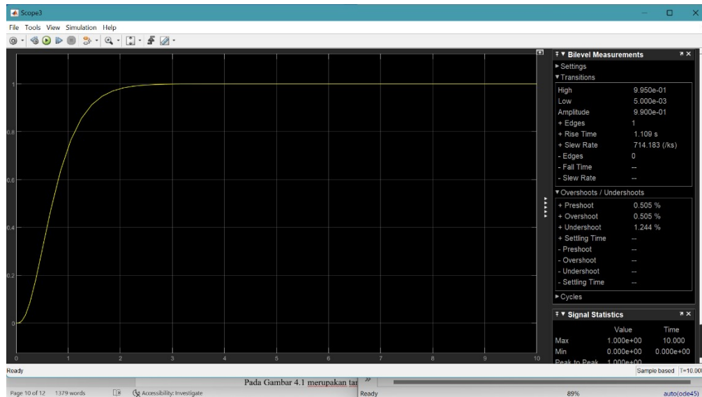
Figure 2. LQR Step Response Display (No Noise)
