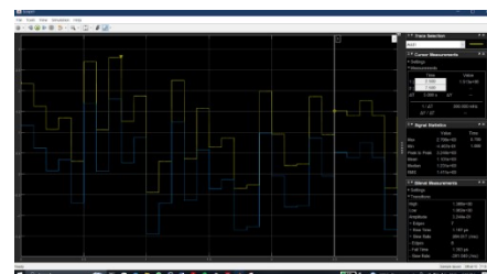
Figure 14. Response Results of Maxon EC-I 40 70Watt DC Motor with LQR Method When Given Noise
