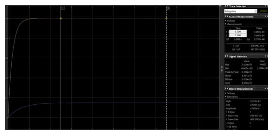
Figure 10. Comparison results of 37-GB500 DC motor response using the LQR method and not using the method
