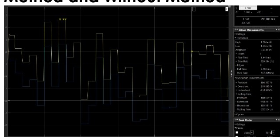
Figure 13. Response results of the MG-16B DC motor using the LQT method when noise is applied
