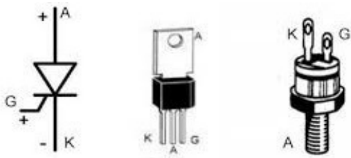
Figure 2. SCR Symbol and Shape
